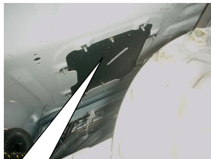
**A "TYPICAL" CHASSIS PTO "ACCESS" HOLE IN THE CAB'S FLOOR...HELPFUL FOR PTO/PUMP "WORK"**
