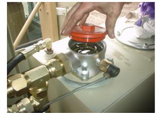
2- Remove the Filter's Top Cover by turning CCW. The Cover's compression spring will be "pushing"...so use your hand over the Red removable polymer cover when it is close to being fully un-threaded to control.
