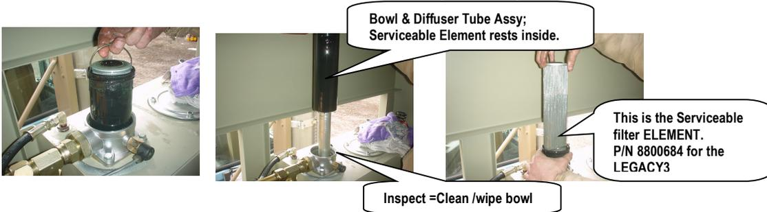
4- Now remove the "old" element. Put it into clean garbage bag so you can later "study" what has been trapped-out of the hydraulic system (can offer "clues" as to the hydraulic system's "health").
