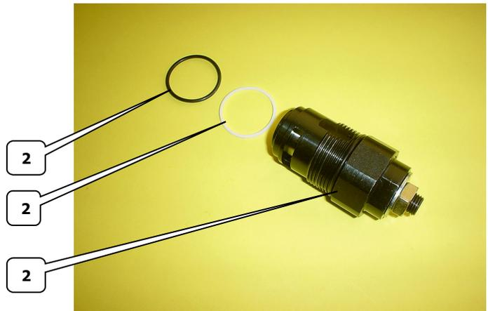
This relief is **NOT** shipped Pre-set to correct Legacy setting! It must be "adjusted". See your Legacy Maintenance manual for "adjusting/ setting" to correct Legacy specification.
