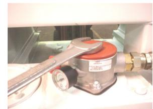
6- Now re-install the filter housings COVER. Snug up with LIGHT-MEDIUM force.
